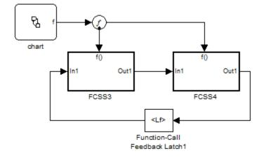
In either case, the latching results in the destination block reading a delayed signal from the previous execution of the source function-call block.
