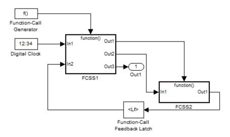
• If a loop involves function-call blocks connected to branches of the same function-call signal, then this block latches the signal at the input of the destination function-call block, and thereby allows it to execute prior to the source function-call block.
